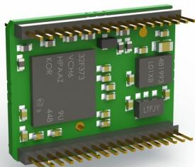
GSV-6 product line provides signal processing for strain gauges on the smallest area. The centerpiece of the GSV-6 is a printed circuit board in the dimensions of 19 x 14 mm. This "GSV 6CPU" provides all necessary functions for the construction of a 1-6 channel of measurement amplifier is ready.
