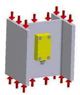
The full pressure strength of the magnets is only achieved on a flat surface. If there are small surface irregularities, air gaps occur between the magnet and the component meaning that the pressure strength is potentially insufficient to compress the strain gauge and the seal. Therefore please check whether the pressure strength of the integrated magnets is sufficient before applying the adhesive. For series DA68e, the following should be observed in particular:
