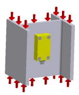
The full pressure strength of the magnets is only achieved on a flat surface. If there are small surface irregularities, air gaps occur between the magnet and the component meaning that the pressure strength is potentially insufficient to compress the strain gauge and the seal. Therefore please check whether the pressure strength of the integrated magnets is sufficient before applying the adhesive. For series DA68e, the following should be observed in particular:
