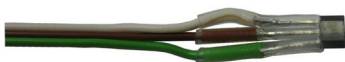
Figure 3: Hall switch HAL501 within the TO92 housing, note the sensitive surface position (should be facing the magnetic south pole)
