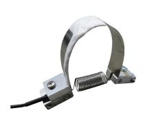
The crack sensor CS40 is used to monitor cracks on structures. Another area of application is the dendrometer, for measuring the perimeter of tree trunks. The path sensor is suitable for single-axis distance measurement for the measuring range of 5mm.
