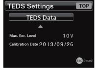
Press the ESC button to exit TEDS data display mode.
