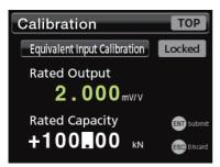
Move the cursor to the digit where you want to show the decimal point, and press the ▲ or ▼ button until the decimal point is shown.
