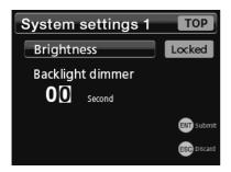
This can be used to set the time until the backlight dims after the last button press (in 1-second intervals up to 60 seconds).
