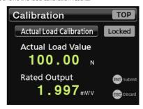
Check the load calibration results. If there are no problems, press the ENT button to confirm them and proceed to the next step.
