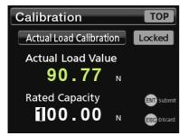
With an actual load applied to the sensor, press the ENT button.
