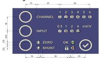
LEDs 1-6: Selected channelLEDs 7-10: Sensitivity of input
