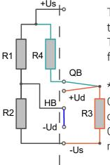
The active strain gauge R3 is connected in 3-wire technology to the terminals Ud+, QB and -Us.
