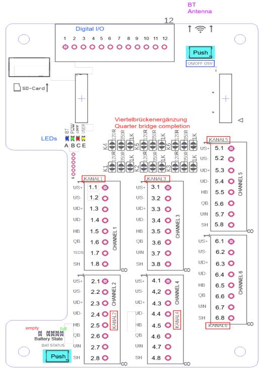
With the push key below, the battery charging state can be checked. With the push key above, the measuring core GSV-6CPU can be powerd on/off (if configured by software).
